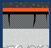
Maintenance of an old asphalt road without regulating layer
