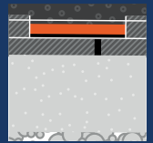
Partial reinforcement of a longitudinal crack with grinding
