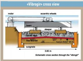
Several specimens were tested with «vibrogir» for different durations, the maximum being 200 hours. Pyramid-puncture tests (NF G 38 019) confirmed that no loss in puncture resistance occured after the vibrogir test; furthermore, no major decrease in either permeability or flow rate was observed.
